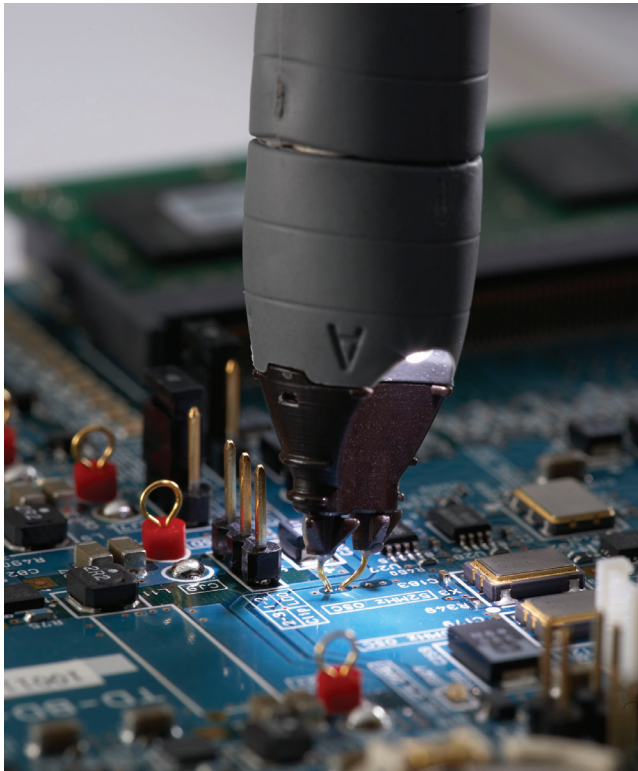
Figure 2. N2750A Series differential probe with browser tip
